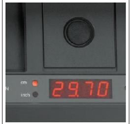
Precise backgauge positioning with the hand crank is very easy due to the digital measurement readout, which can be switched over from mm to inch.
