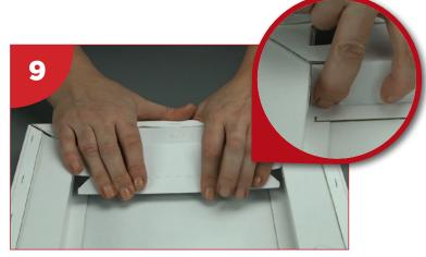
Press down, (checking you're happy with your corners) hold in place and then roll inner frame edge downwards, clicking locking tabs into position.
