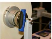
The mandrel has a hinged support and provides a handy storage for the T-bar Allen key.
