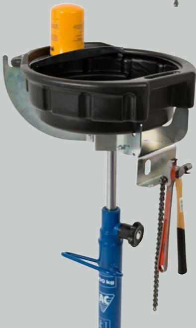
The bracket has allocated space for tools, screws and small parts
