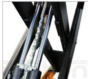
Mechanical locking mechanism
