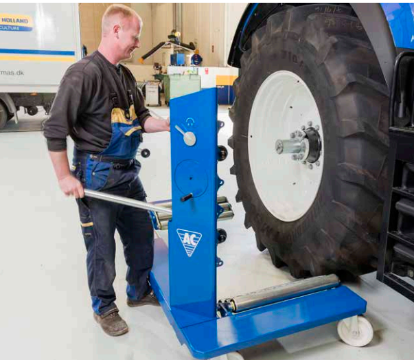
Rotate the wheel to align the studs perfectly when re-fitting the wheel
