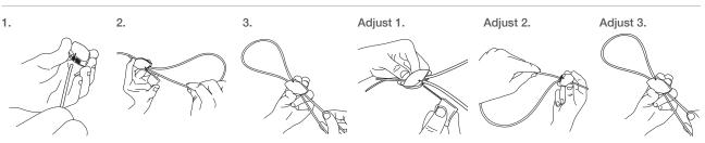
Ensure a minimum 75 mm of tail wire exits the hanger.
