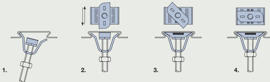
1. Pre-assemble the bracket and Multi-Nut (flat surface facing up) onto the threaded rod and insert one side of bracket into re-entrant channel of decking.
