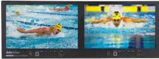
TLM-102 is a dual 10.1" rack-mounted monitor unit, designed for broadcast, video production and AV users. It features a 4RU rack design with SDI & HDMI in/outputs. It offers a various of mounting methods for live monitoring, integration into portable production units and use in and OB vans.
