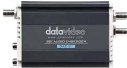
DAC-91 is an audio embedder that allows users to embed 2 channels of analog audio into an SDI video signal. It features 3G/HD/SD-SDI to support up to 1080p/60 video, automatically detecting and switching between different formats, and provides mini XLR and RCA audio connectors for inputting embedded audio. The audio box also has audio level adjustment.
