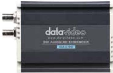
DAC-90 is an audio de-embedder box that allows users to de-embed 16 analog audio signals (4 at a time) from SDI video signal. It features 3G/HD/SD-SDI to support up to 1080p/60 video, automatically detecting and switching between different formats, and provides 4 mini XLR audio connectors for outputting analog audio to audio devices such as, recorders, switchers, and audio mixers. The Audio box also has SMPTE and EBU settings.
