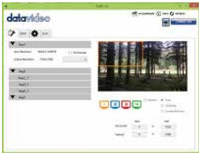
When we feed a 4K source into TWP-10, the layout will be set to 2x2. In this setting page, users can see the input source resolution and monitor the frame rate and select the requested output resolution.
