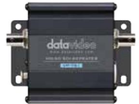
The VP-781 HD/SD-SDI with Intercom repeater is designed to cascade CB-46/ 47/ 48 cables, extending the transmission range of video, audio and intercom signals. To connect VP-633 that the VP-781 is able to extend video up to 200M.
