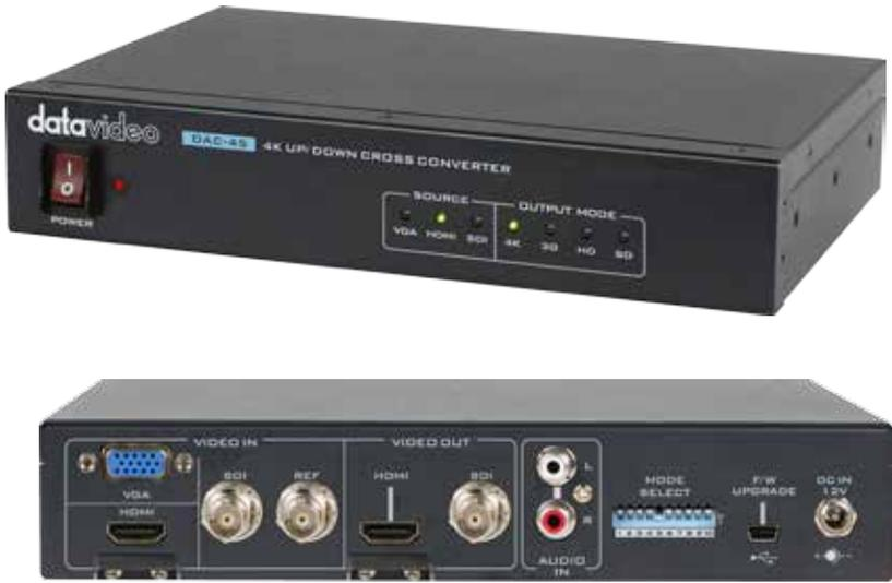
DAC-45 is an auto-sensing 4K up/down/ cross converter. This product seamlessly converts VGA, HDMI and SDI to 4K or 1080P HDMI and SDI. There is additional RCA audio embedding, to embed a stereo signal to the HDMI or SDI output.
