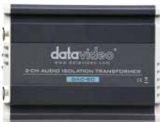
DAC-80 is designed to remove hum and buzz created by ground loops. Voltage differences between different pieces of equipment cause small AC power currents to flow within the shield of audio cables. Capacitance issues can also introduce small current flows within the cable shield. Both problems will create hum in audio signals. DAC-80 delivers the clean audio signal you need, yet remains transparent within the production chain.
