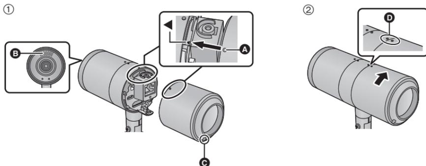
**1** Align the mark ◀ on the camera body with the mark **A** on the rear cover and insert it.
