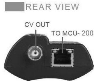
This unit allows you to operate the functions of the camera up to 300m away with the MCU-200 unit.
