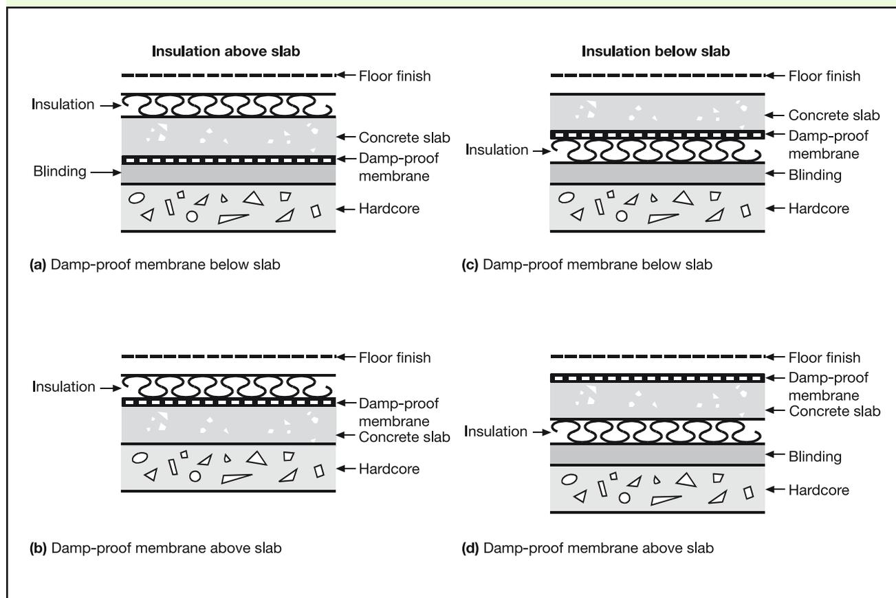
**4.8** A membrane below the concrete could be formed with a sheet of polyethylene, which should be at least 300 $\mu$ m thick (1200 gauge) with sealed joints and laid on a bed of material that will not damage the sheet.
