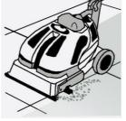
STEP 3. Set solution release rate on the machine and scrub
