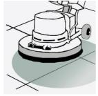
STEP 3. Scrub surfaces with a rotary scrubber to release cement & salt residues.
