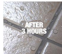
Test area with a little water and apply another coat if water is absorbed.
