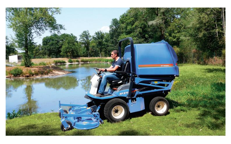
A great value out-front rotary mower utilising a tractor chassis for superb durability. With a choice of either 30hp or 36hp engines, these machines guarantee safe and reliable service on difficult terrain, while the comfort enables a higher volume of work to be carried out for long periods with minimal stress to the operator.
