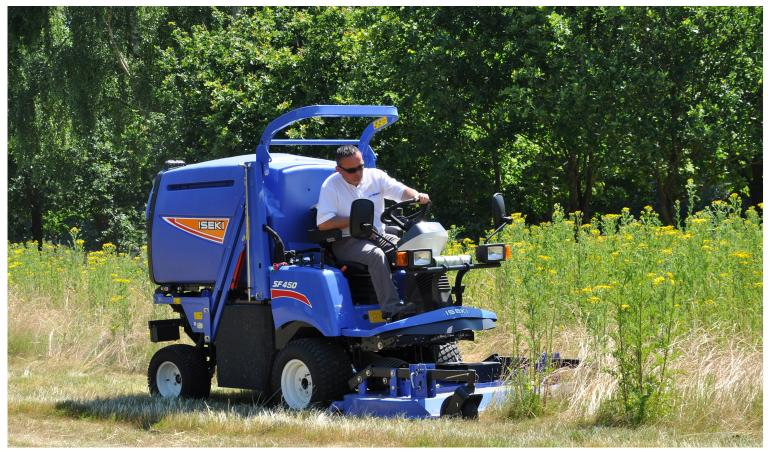
The ISEKI SF450 is a large capacity centre collect rotary mower. Fitted with a 1.52m (60") deck and a 1300 litre hopper, the SF450 is highly productive. The high torque 35kW (46hp) engine ensures ample performance to cut and collect lush grass growth and maintain speed. With muching plate supplied, the SF450 is an extremely versatile mower.
