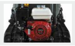
**ENGINE** The Carry 105 mini-dumper has a Honda 4.7 kW rpm petrol engine with pull-cord starter.
