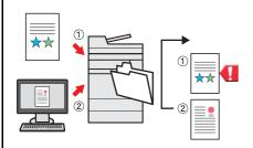
When paper empty error occurs at the cassette by specifying the special paper size or type, the machine skips the error job and perform the next job
