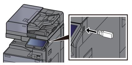
When the machine reads the USB drive, "USB Drive is recognized. Displaying files. Are you sure?" may appear. Select [Yes] to display the USB Drive screen.
