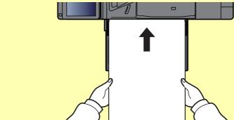
• After printing starts, catch the paper when it is output so that it does not fall. When using the inner tray as the output location, do not stand up the stopper.
