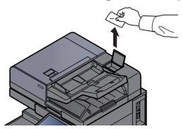
Clean the slit glass surface and the reading guide.
