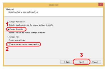
Selecting the [Overwrite settings on target device] checkbox will overwrite the machine's Address Book from entry No.1.
