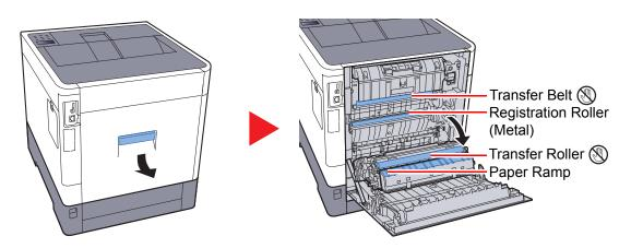
Wipe away the paper dust on the registration roller and the paper ramp using the cloth.
