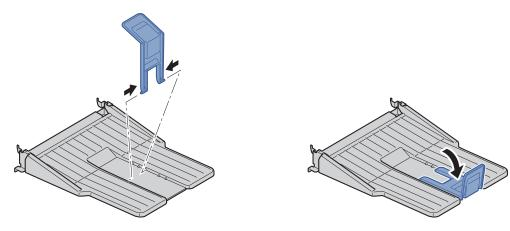
2 Install the rear tray on the rear of the machine.
