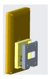
• metal plate for mounting on <u>Vesa</u> (Video Electronics Standards Association) standard supports
