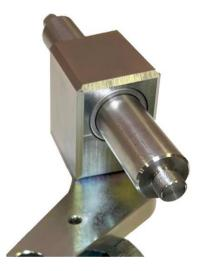
Step 3: Insert the Adjustable Tube Clamp into the Main Plate
