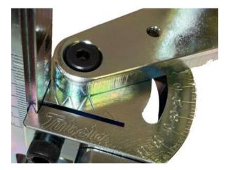
When a compound angle is required the V-Pads and both scales can be adjusted to suit the required angles, please ensure both the tube and all locking bolts are firmly secured before operating the Piranha Notcher.
